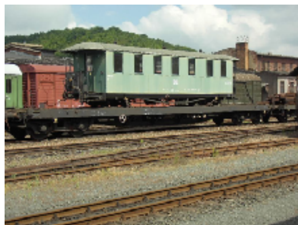
Coming or going? A narrow gauge carriage sits on a standard gauge wagon waiting for attention.
