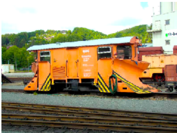
An interesting feature. A double ended self propelled snow plough!
